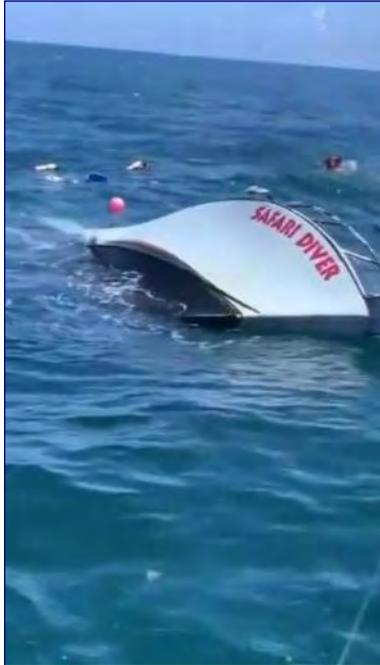
Company's Black Pearl, was told by a crew member that the vessel's propeller fouled the mooring line the captain had attached to the wreck they intended to dive. The rotating prop managed to winch the vessel's stern underwater before the captain could grasp what was happening and stop the engine. The hull quickly filled with water and the vessel went down within minutes. ★
